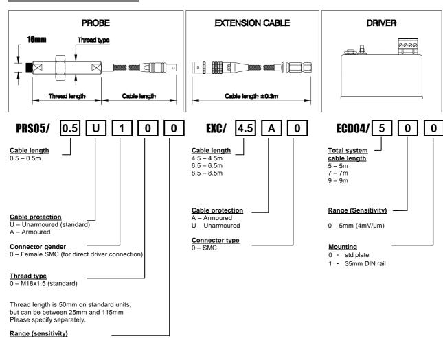
Note: Total system lengths must add up to 2, 5, 7 or 9m (2m systems cannot include extension cables). Probe system length may be up to 0.7m longer than stated.
