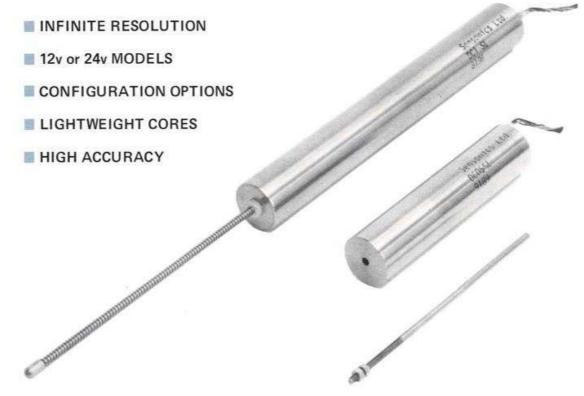
The DM series of DC/DC linear transducers cover the range ± 2.5mm to ± 50mm and are intended as a general purpose instrument. As with all other Sensonics LVDT's they are robustly housed with impregnated coils and internally potted so that they are suitable for use in the majority of industrial applications.
