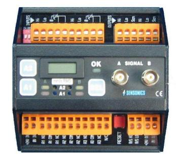
Input: 2 x Eddy Current Probes & Drivers 200mV/mils (8mV/um) as standard.
