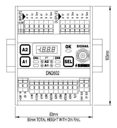
Input: 2 x Eddy Current Probes & Drivers 200mV/mils (8mV/um) as standard.
