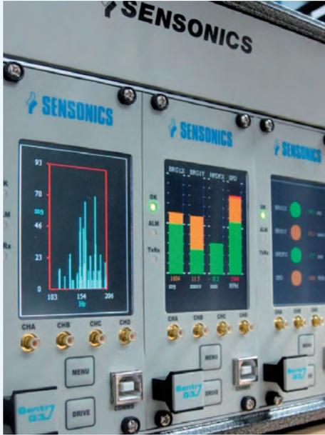
An upgrade of the intuitive display to a colour LCD also provides additional features not possible with the previous generation, such as the display of all measurement values and alarm colour coded bar graphs. The vibration spectrum can also be viewed at a touch of a button; combined with channel parameter trending displays, these additional facilities will prove invaluable to instrumentation engineers in evaluating and keeping track of critical rotating plant performance.
