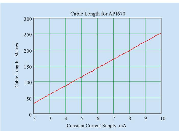
If we translate this into acceleration and look at the effect of different value current loops (diodes), the potential limitations in the dynamic range of the measurement system can be seen.
