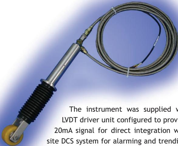
The instrument was supplied with an LVDT driver unit configured to provide a 4-20mA signal for direct integration with the site DCS system for alarming and trending.
