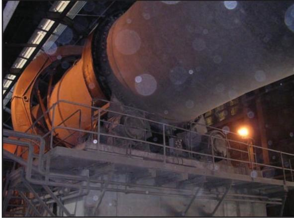
Kiln with support and drive structure
