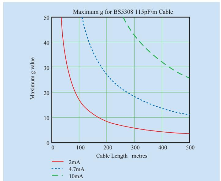
ATEX applications with accelerometers mounted within a hazardous area are limited by the overall circuit capacitance seen by the safety barrier at the interface between the safe and hazardous areas.
