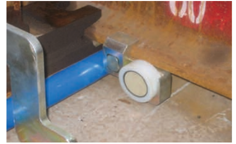
Probe positioned on fixed rail - opposite switch rail target
