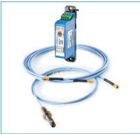
The cable system incorporates snap lock connectors which require no torqueing and provide a shake proof solution important for heavy industrial applications. The double screened cable offers robustness in combination with high immunity to interference and optional stainless steel convoluted armour is available for applications or environments where cable protection is paramount.
