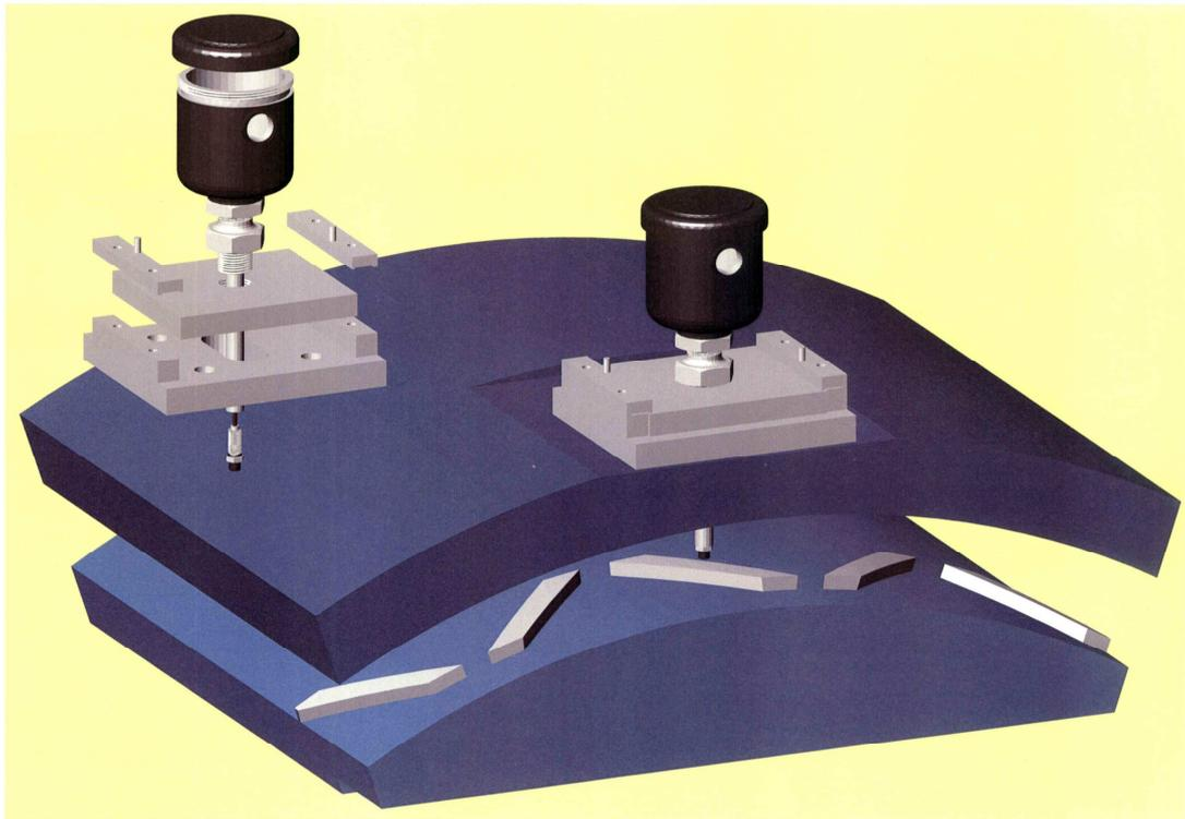
*Typical probe sliding bracket and clamp arrangement*
